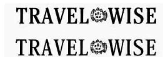
Figure 2: Acrobat uses the original font metrics and a multiple master font to preserve the characteristics of the original. On top is the original ITC Cheltenham® Condensed Bold font; below is the Acrobat substituted font, Adobe SerifMM.
